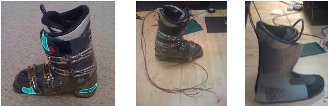
Figure 3 Left: sensor placement. Center: Fully instrumented boot. Right: Liner with sensors.
