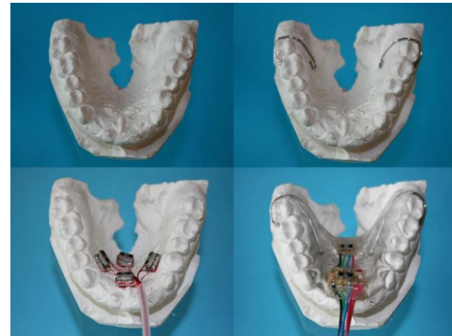
Figure 3: Process steps for fabricating a tongue input device
